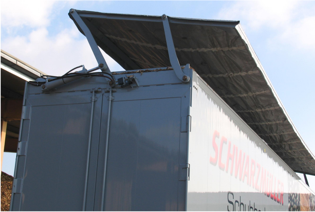
OPTIONAL: Hydraulic folding roof with all-round frame and plastic tarpaulin
